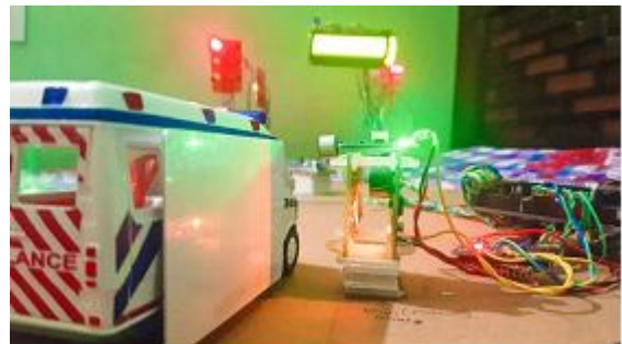
Fig. 7: Ambulance approaching RFID 1 & Sound Sensor
