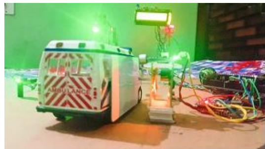
Fig. 8: RFID Reader & Sound sensor activated by RFID Tag & Ambulance siren frequency
